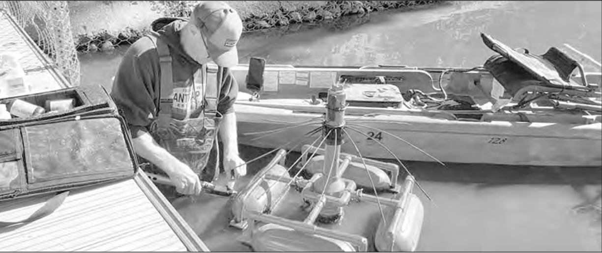
George Klug deploying a WQ3D water testing device in Fergus Falls' Lake Alice.
